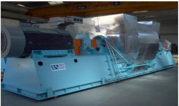
Structure and the Phone Control of the Fax Notestation of E-mail www.control of Web FAN DATA DESIGN FAN TYPE: BCSN 542 DWDI **ARRANGEMENT: 7 DWDI -DOUBLE DRIVER** SERVICE: COMBUSTION AIR FAN **BLADES TYPE: HOLLOW** AIRFOIL FLUID HANDLED: FRESH AIR FLOW RATE: 300.000 M3/H STATIC DIFFERENTIAL PRESSURE: 900 MMWG **SPEED: 1780 RPM INSTALLED POWER: 1100 KW** SITE: TASNEE **PETROCHEMICAL COMPLEX.** AL JUBAIL
