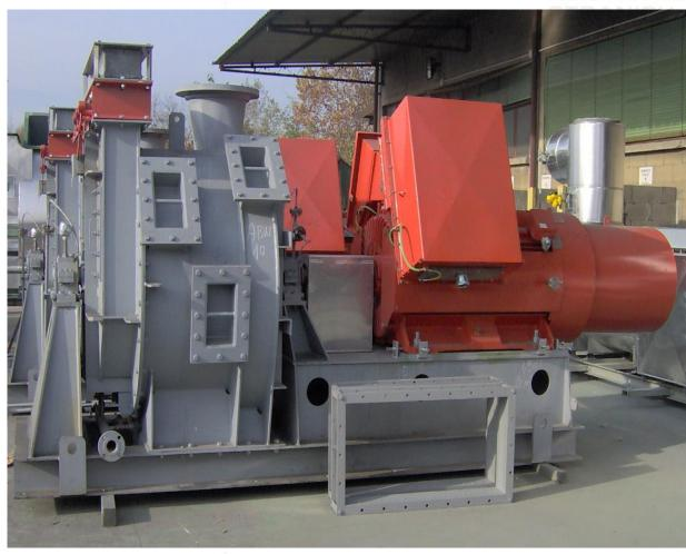
FAN DATA DESIGN FAN TYPE: ABN 10 TS (THREE STAGES BLOWER) **ARRANGEMENT: 7** SERVICE: COMBUSTION **AIR BLOWER BLADES TYPE: BACKWARDLY INCLINED** FLUID HANDLED: FRESH AIR FLOW RATE: 13,000 KG/H STATIC DIFFERENTIAL PRESSURE: 0.9 BAR G **SPEED: 2990 RPM INSTALLED POWER: 350** KW SITE: QAPCO EP2-QATAR
