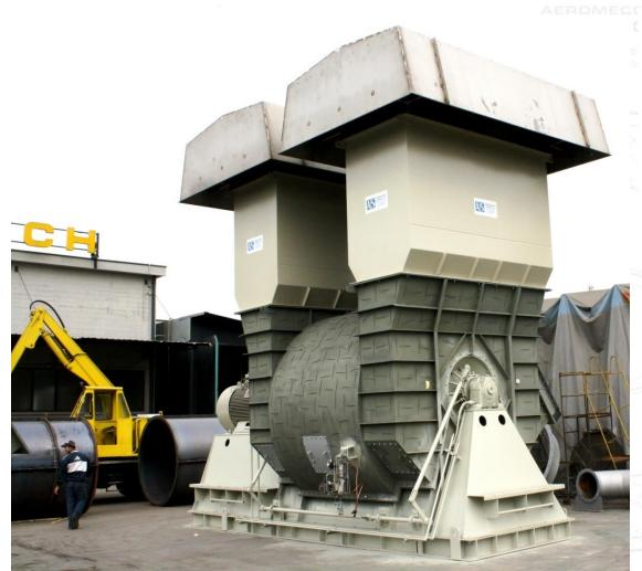
FAN DATA DESIGN FAN TYPE: BCSN 660 DWDI ARRANGEMENT: 7 DWDI SERVICE: COMBUSTION AIR FAN BLADES TYPE: HOLLOW AIRFOIL FLUID HANDLED: FRESH AIR FLOW RATE: 300,000 M3/H STATIC DIFFERENTIAL PRESSURE: 600 MMWG SPEED: 985 RPM INSTALLED POWER: 550 KW SITE: SHELL PEARL PROJECT (QATAR)
