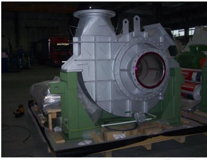
FAN DATA DESIGN FAN TYPE: TSP-90 **ARRANGEMENT: 8 SERVICE: BOOSTER** FAN **BLADES TYPE: RADIAL BLADE** FLOW RATE: 32,400 M3/H STATIC DIFFERENTIAL PRESSURE: 475 MMWG **SPEED: 2950 RPM INSTALLED** POWER: 110 KW SITE: CBDC
