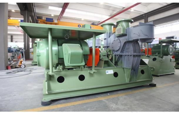
FAN DATA DESIGN FAN TYPE: ABD 84-DS **ARRANGEMENT: 7** SERVICE: EXHAUST **BLOWER FOR RTO BLADES TYPE: BACKWARD CURVED** FLOW RATE: 2,000 M3/H STATIC DIFFERENTIAL PRESSURE: 4000 MMWG **SPEED: 3560 RPM INSTALLED POWER: 90** ĸW SITE: RABIGH II
